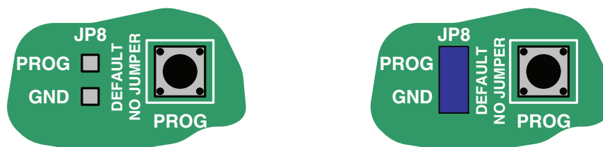
a) No Jumper: FPGA Operational (default)
